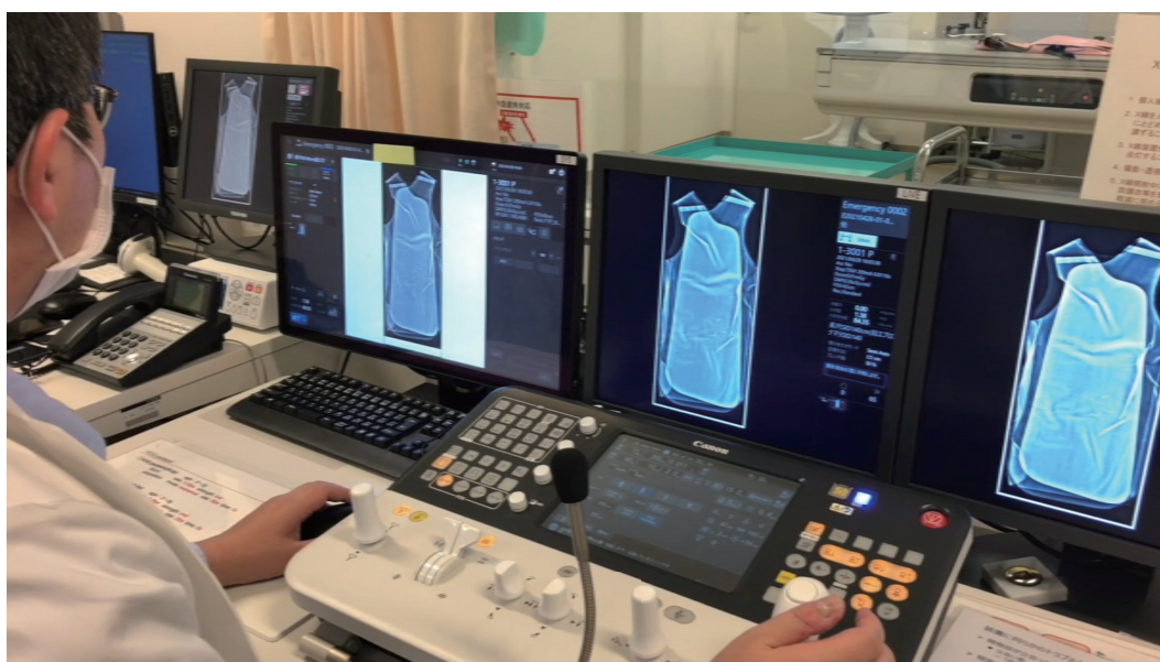
Figure 10: Stitching radiography of X-ray protective equipment
